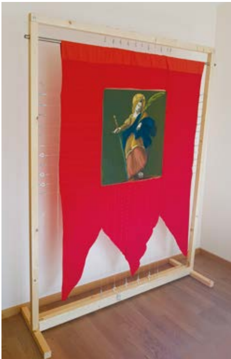
12. Experiment no 2. The banner with a double-sided painting ( St. Catherine of Alexandria ) stretched with spring system, photo by Milda Tičkaitė, 2021
