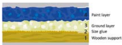
2. Diagram of a cross-section of the polychrome sculpture, illustration by Angela Caira, 2021
