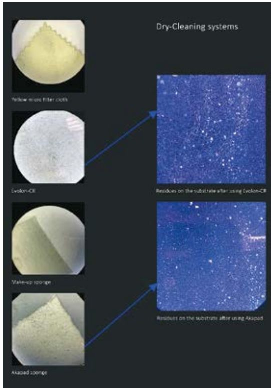
8. The dry cleaning systems, photos by Anastasiya Serdyukova, 2021
