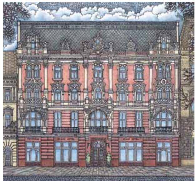
7. Use of coloured plaster in the façades of Late Historicism (Grand Hotel). Drawing by the author, 2016
